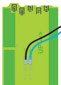
Example of corrected FRESH TOP sender programming (GRY or BLK tab cut by mistake)
