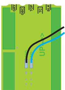
Example of corrected GRAY SINGLE or BOTTOM sender programming (BLK tab cut by mistake)
