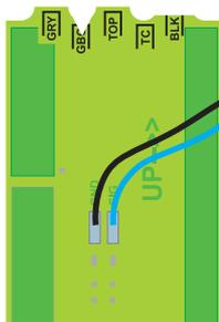
Example of corrected FRESH SINGLE or BOTTOM sender programming (TOP tab cut by mistake)
