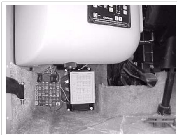
Fig. 10-18 COMMANDER FUSE PANEL
