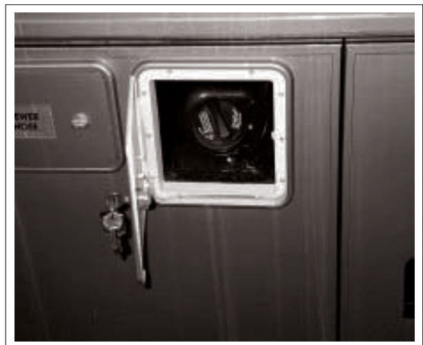
Fig. 10-8 GENERATOR REFUELING (GAS ONLY)
